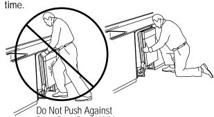
Do Not Push Against Front Door Panel With Knee. Damage to The Door Panel Will Occur.
